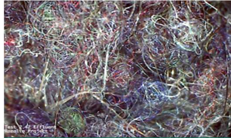
Photo shows a 3 mm (0.1 in) section of microfibers filtered from drain water of standard load of laundry magnified 120 X
